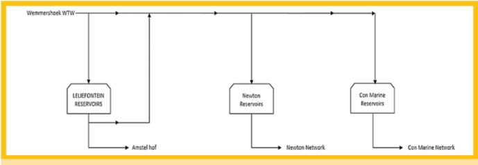
FIGURE 1: Existing Network Under Gravity Flow
