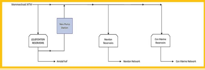
FIGURE 2: New Leliefontein Booster Pump Station Addition to Existing Gravity Network
