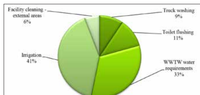
FIGURE 3: Distribution of the daily 2 nd class water demand for an example of an industrial development with onsite WWTW
