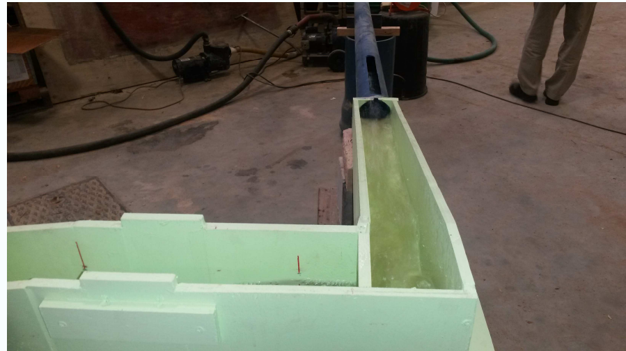
Flow in 3D Model of 90° Stilling Basin
