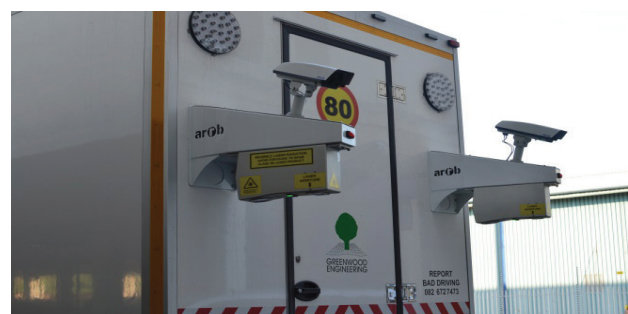
FIGURE 7 The ACD system installed at the rear of the trailer measures 4000 points (combined) across the lane. It also houses the rear facing asset cameras
