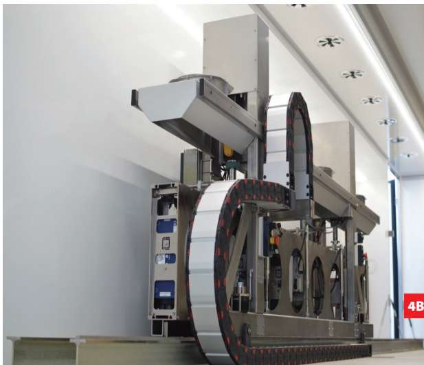
FIGURE 4A AND 4B The beam which houses the Doppler laser sensors
