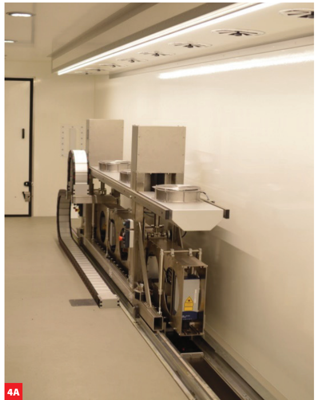
FIGURE 4A AND 4B The beam which houses the Doppler laser sensors
